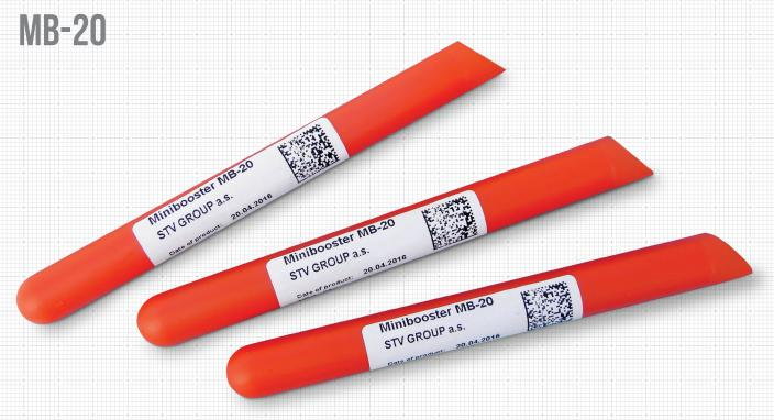
The Minibooster MB-20 is an industrial explosive, which consists of a plastic shell filled with plastic explosive based on RDX and PETN. Miniboosters are designed for initiating industrial explosives, particularly to carry out blasting operations on the surface and in non-explosive underground environment.
